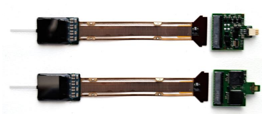
Figure 33: Correct way to plug the flex in the ZIF connector. Top: front side dock 1, Bottom: back side dock 2
