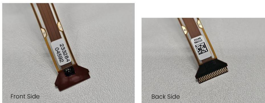
Figure 7: Left: Label with unique probe ID attached to ZIF area front side. Black epoxy covers the EEPROM. Right: ZIF area back side with metal contact pads and unique probe ID and QR code.
