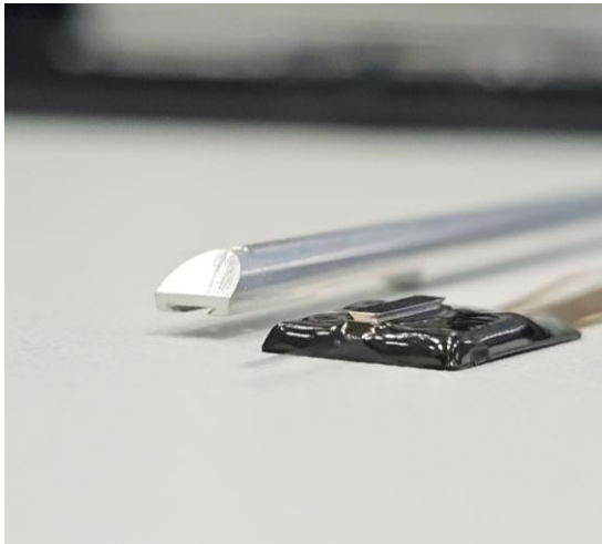
Figure 8: Neuropixels 2.0 quad base multishank probe with Cap and the dove tail holder (HOLDER_2000_C)
