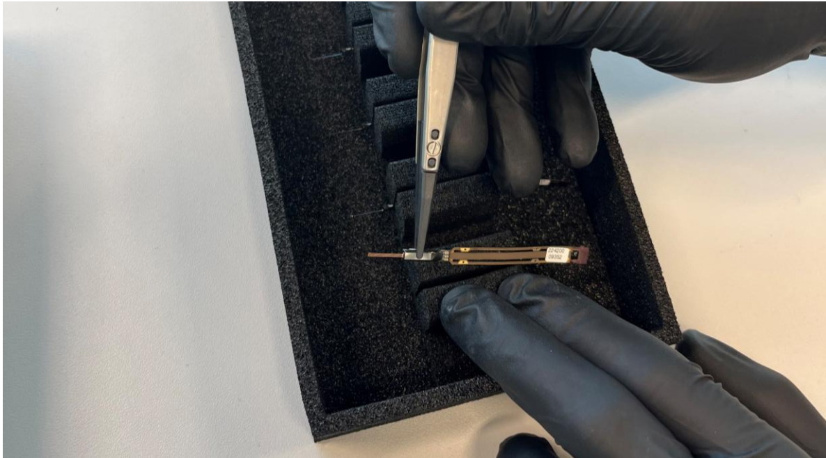
Figure 45: Removing the probe from the foam by clamping the base with tweezers.
