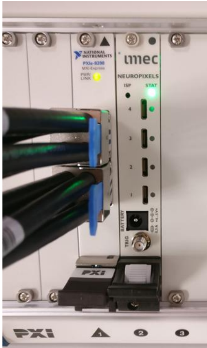
Figure 23: Global status LED of the PXIe acquisition module switching from red to green after correct installation.
