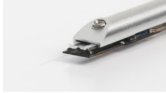
Figure 8: Neuropixels 1.0 HD probe mounted on the dedicated dove tail holder (HOLDER_1000_C)
