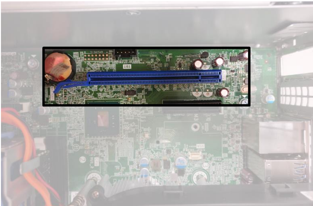
Figure 22: PCIe x16 slot on the PC motherboard.
