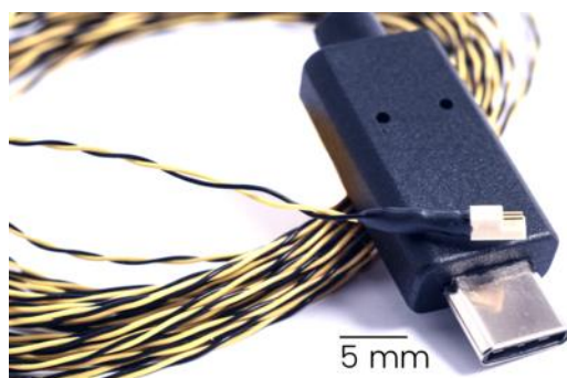
Figure 12: Twisted-pair interface cable with Omnetics-to-USB-C termination.
