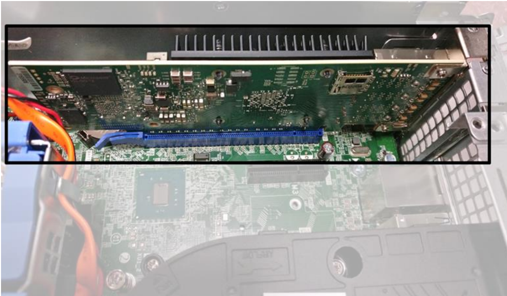
Figure 23: NI PCIe-8398 board plugged into the PC.
